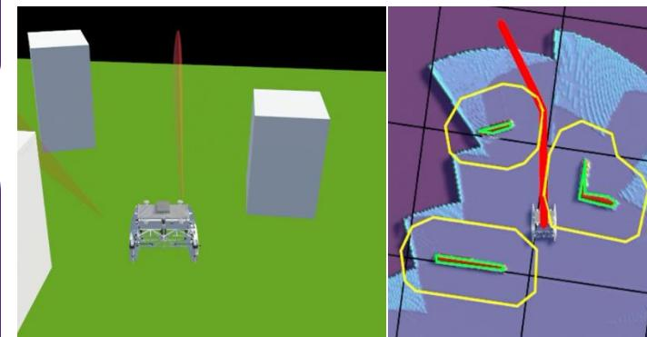
Adaptive scanning outperforms a simple speed-adjusted strategy in 9/10 randomly generated obstacle courses, improving average no-intervention rate from 0.411 to 0.7.
